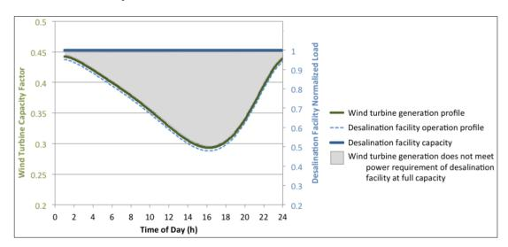
The economic and geographic feasibility models evaluate profitability considering annual production. The capacity of the wind turbine considered ( $C_{WT}$ , in units of kW) is determined based on the power requirement of the desalination facility for desired generation (P, in units of kW) and the peak of the average wind turbine capacity factor daily profile ( $CF_{WT,Peak}$ , a dimensionless ratio), as in Equation (5):
