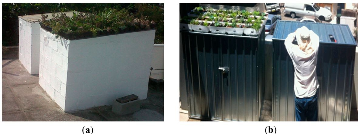
Figure 2. Housing thermal experiments. (a) Rio de Janeiro; (b) Sydney.
