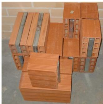
**Figure 12.** Clay bricks including PCM macro-capsules [61].
