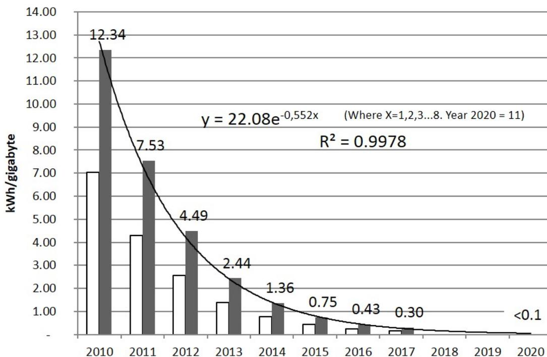
**Figure 3.** Development of energy efficiency of transmitted mobile data (kWh/gigabyte) in Finland during 2010–2017. Grey bars represent estimated consumption for production networks and white bars for base stations only. Exponential trends ( $y = y(x)$ ) until 2020 were estimated by means of least squares fit using the data in the grey histogram. X in these equations refers to numbers 1 to 8; and 11 corresponding to years from 2010 through to 2017; and 2020.
