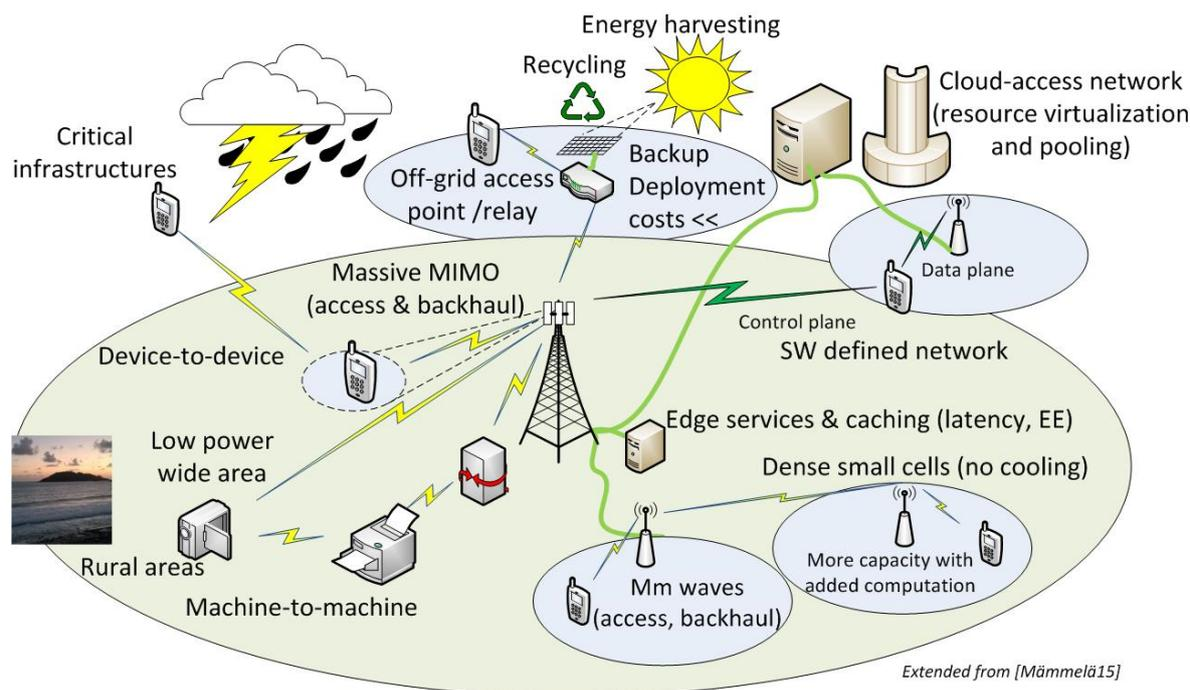
**Figure 4.** 5G techniques have a clear impact on energy efficiency (EE). (Source: [23], published with permission from the author.)
