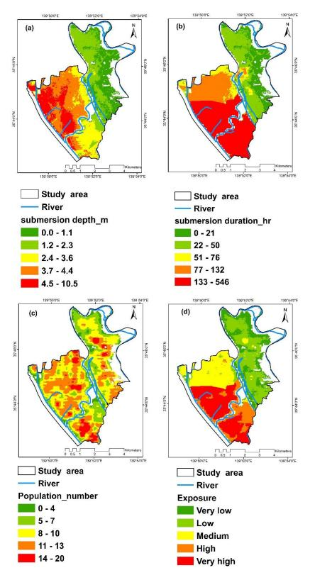
**Figure 3.** Exposure to flood: (a) Submersion depth distribution; (b) submersion duration distribution; (c) population distribution; (d) exposure.
