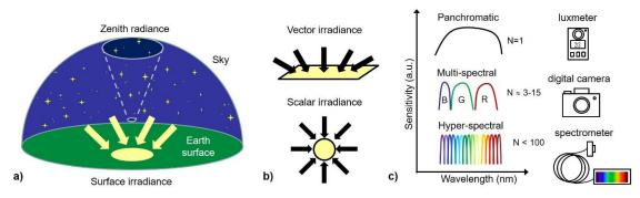
**Figure A1.** Schematic drawing of different radiometric parameters: (**a**) geometry of sky and zenith radiance and surface irradiance measurements; (**b**) vector and scalar irradiance; (**c**) different spectral bands: single (panchromatic), multiple (multi-spectral), and full spectrum (hyperspectral) (after Reference [173]).
