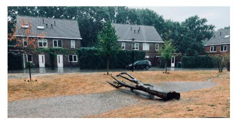
**Figure 6.** Example of temporary rainwater conservation and infiltration in "wadi's" on slopes in Ede, The Netherlands (picture Koen Claassen).
