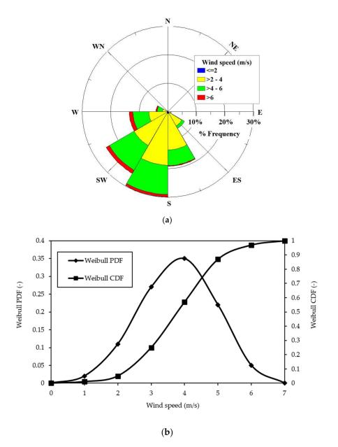
Figure 4. Wind conditions at Deokjeok-do Island (a) Wind rose (b) Weibull plot [22].
