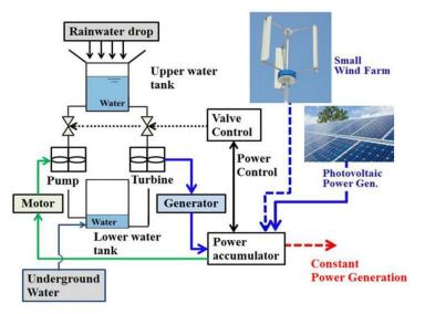
Figure 1. Conceptual design of a typical hybrid renewable energy system (HRES) [22].
