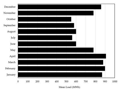
Figure 3. Monthly electric load at Deokjeok-do Island [23].
