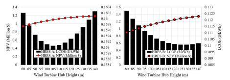
Figure 9. Effect of wind turbine hub height on the economics of both systems.
