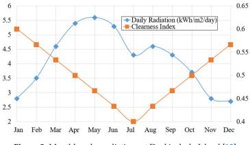
Figure 5. Monthly solar radiations at Deokjeok-do Island [13].
