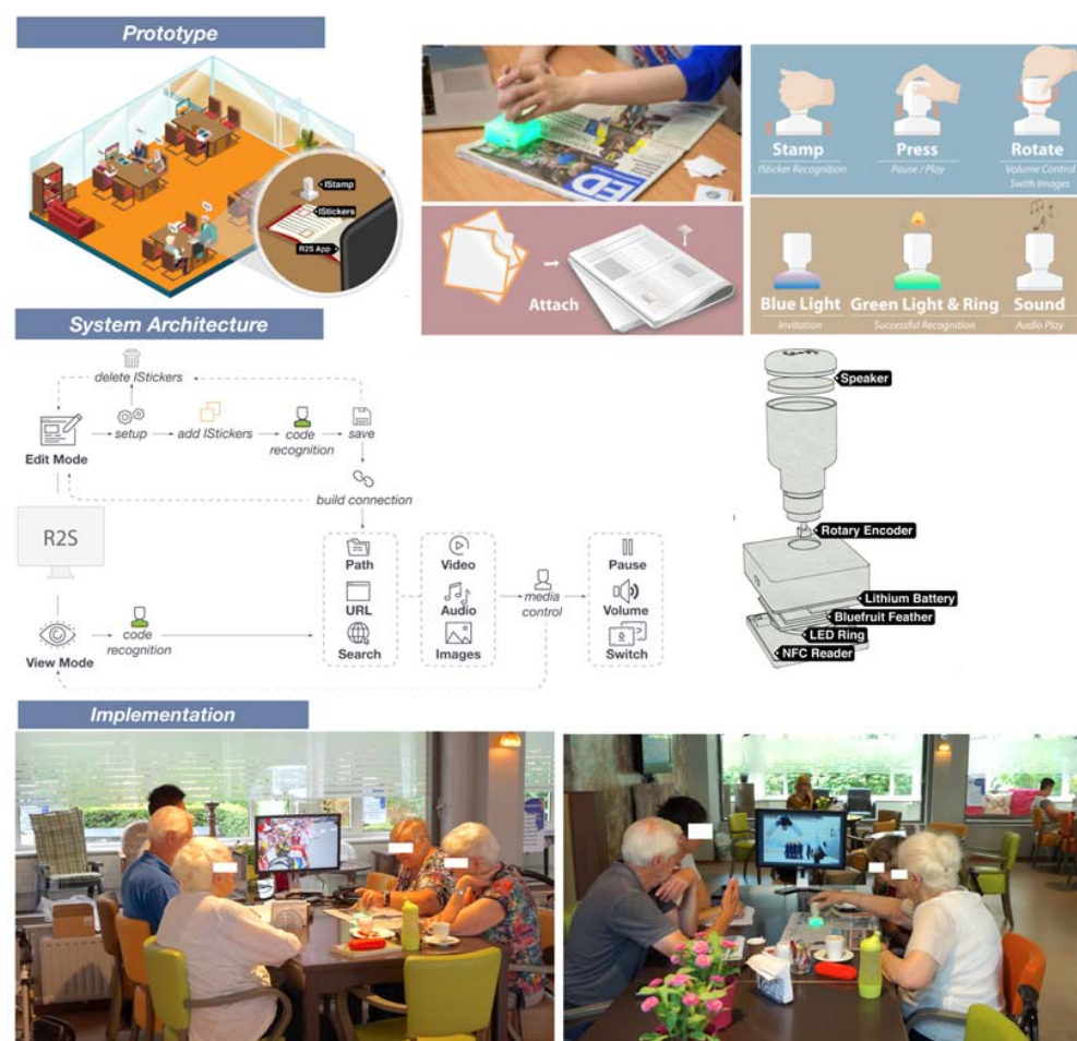
Figure 8. The prototype, system architecture, and implementation of READ2SHARE.
