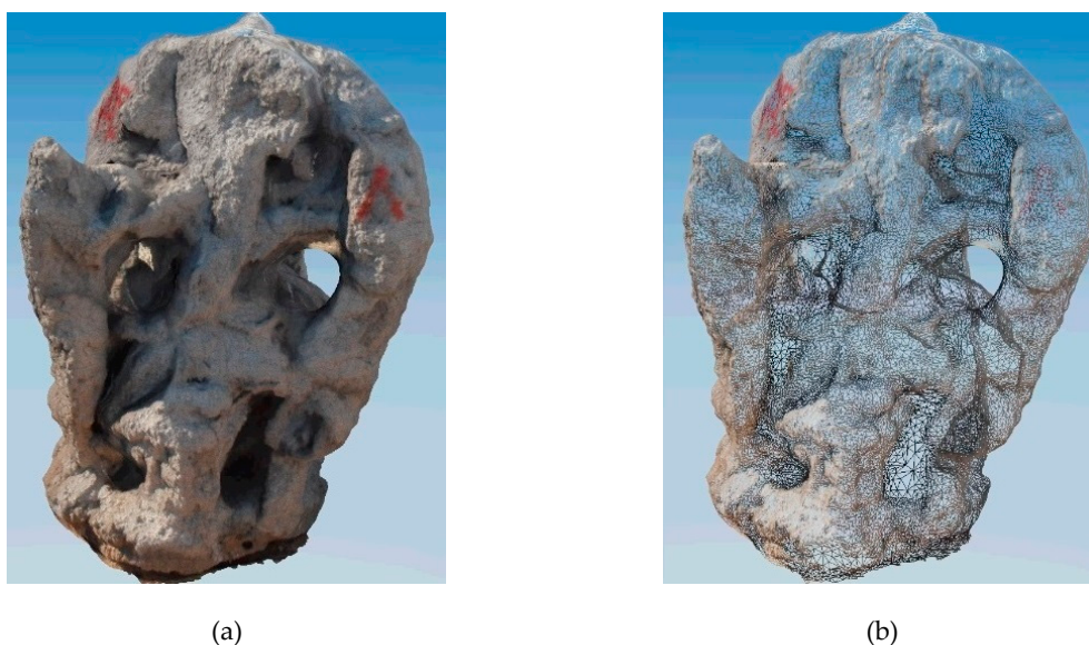
Figure 5. (a) Photo of an artificial reef unit. (b) The 3-D generated mesh for the respective artificial reef unit.
