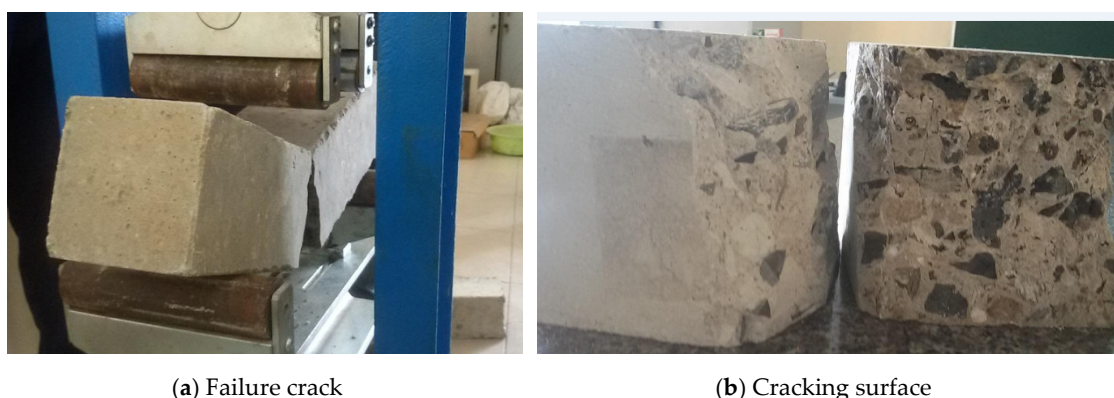
Figure 11. Typical crack under 4-PBT using 100 \times 100 \times 300 mm specimen of CSCs.
