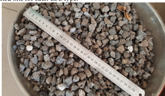
(a) Coarse steel slag used in concrete
