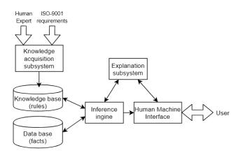
Figure 5. System architecture.
