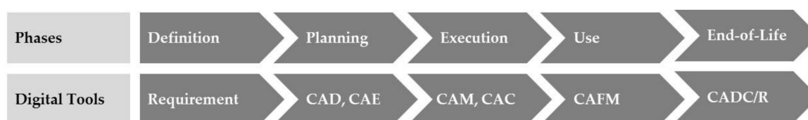
Figure 2. Construction process and digital tools (CAD: Computer Aided Design, CAE: Computer Aided Engineering, CAM: Computer Aided Manufacturing, CAC: Computer Aided Construction, CAFM: Computer Aided Facility Management, CADC/R: Computer Aided Deconstruction/Recycling).
