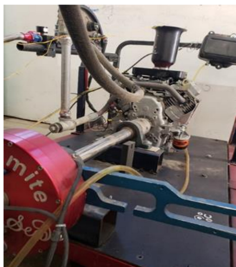
Figure 1. Engine connected to the hydraulic brake.
