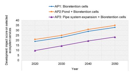
**Figure 5.** Development impact of selected blue-green and grey infrastructure combinations on ecosystem service delivery overtime.
