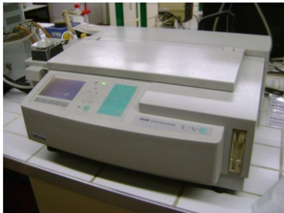
Figure 4. UNICAM UV/VIS Spectrophotometer.
