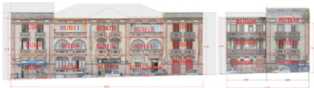
Figure 10. Reggio Calabria. Urban Block #102. Cadastral parcel n. 236. Real estate urban units (subalterni catastali) from Urban Building Cadastre. Garibaldi main street (today: Amendola boulevard) front/façade. Orthophotography. Scale 1: 500. Source: authors’ survey.
