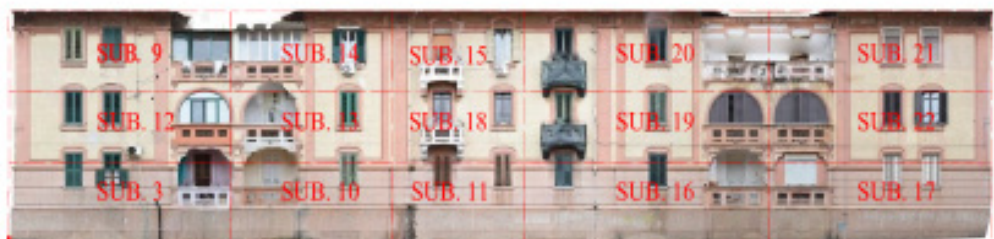
Figure 14. Reggio Calabria. Urban Block #102. Cadastral parcel n. 144. Real estate urban units (subalterni catastali) from Urban Building Cadastre. Minniti Street front. Orthophotography. Scale 1: 500. Source: authors' survey. Minniti Street elevation\front.
