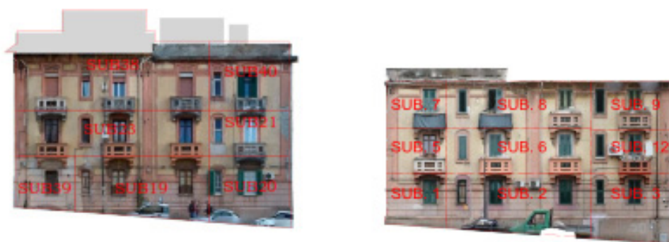
Figure 11. Reggio Calabria. Urban Block #102. Cadastral parcels: (left) n. 236, (right) n. 144. Real estate urban units (subalterni catastali) from Urban Building Cadastre. Mattia Preti Street front. Orthophotography. Scale 1: 500. Source: authors’ survey.
