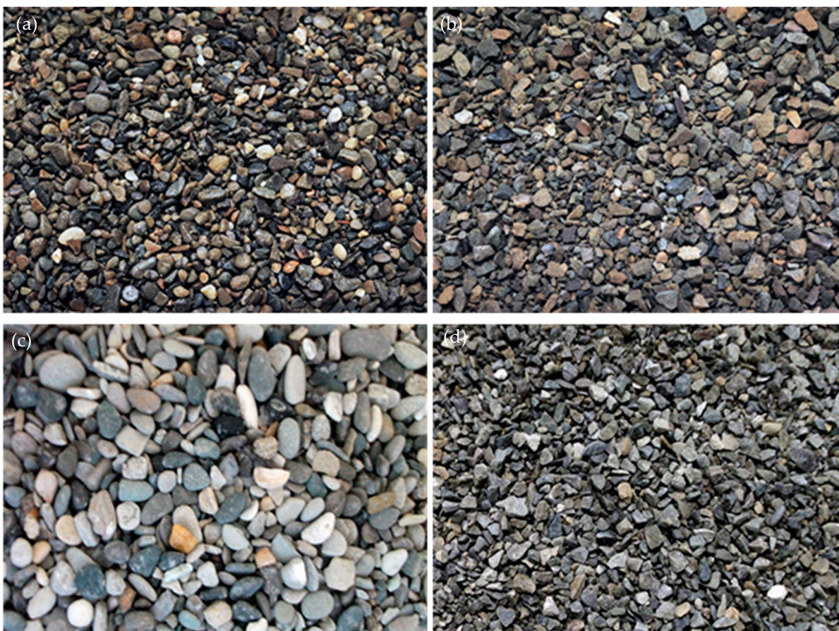
Figure 1. Examples of natural gravel and grit aggregates: (a) gravel 2–8 mm from ZEK Strzegocice II, (b) grit 2–8 mm from ZEK Strzegocice II, (c) gravel 8–16 mm from ZEK Ostrów, and (d) grit 8–16 mm from ZEK Ostrów. Own study based on [44].
