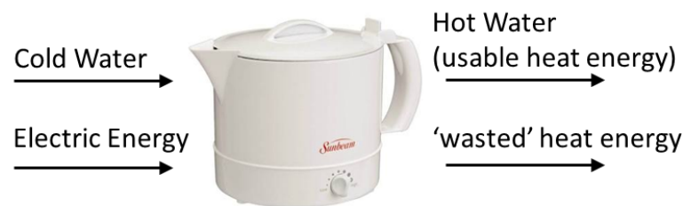
Figure 2. The electric water kettle—a simple energy system that uses electric energy to provide hot water.
