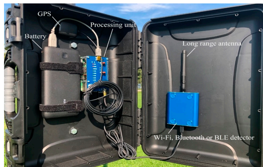
Figure 1. A signal scanner used in the research and its internal components.
