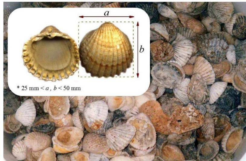
**Figure 1.** Seashell sample used in the present study (before crushing), size and configuration. The \* is explaining the dimensions of the applied seashell.
