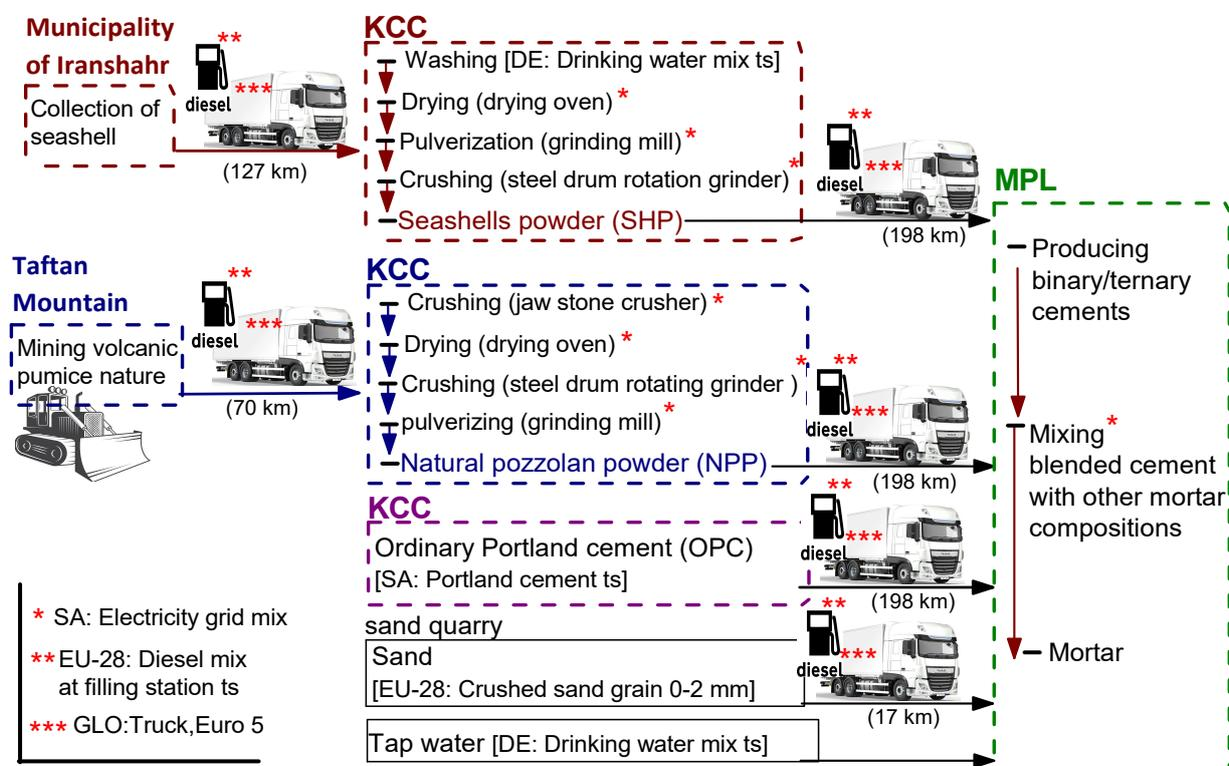
**Figure 2.** Processes considered in the environmental analysis of the mortars made of different blended cements developed in this study.
