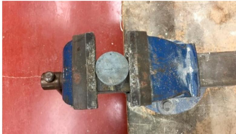
**Figure 1.** Cracking of specimens using screw jack.
