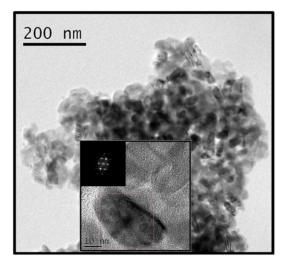
**Figure 4.** Nanoparticulated aggregate containing Si-Al-K-O-amorphous phases associated with anatase and Ti-NPs, with an FFT-containing magnification for an isolated anatase particle.
