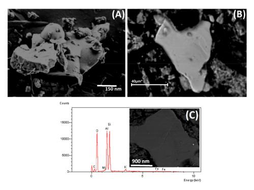
**Figure 3.** Principal particles and minerals detected in the warehouse yards. **(A)** Amorphous compounds; **(B)** Chlorite; **(C)** Illite and EDS containing trace elements.
