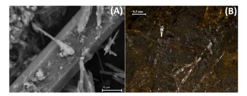
**Figure 5.** Hydrated phases formed with greater abundance during rainy and/or higher humidity periods. (**A**) Analysis of pickeringite by FE-SEM; (**B**) Photo of gypsum using magnifying glasses attached to a Nikon digital camera.
