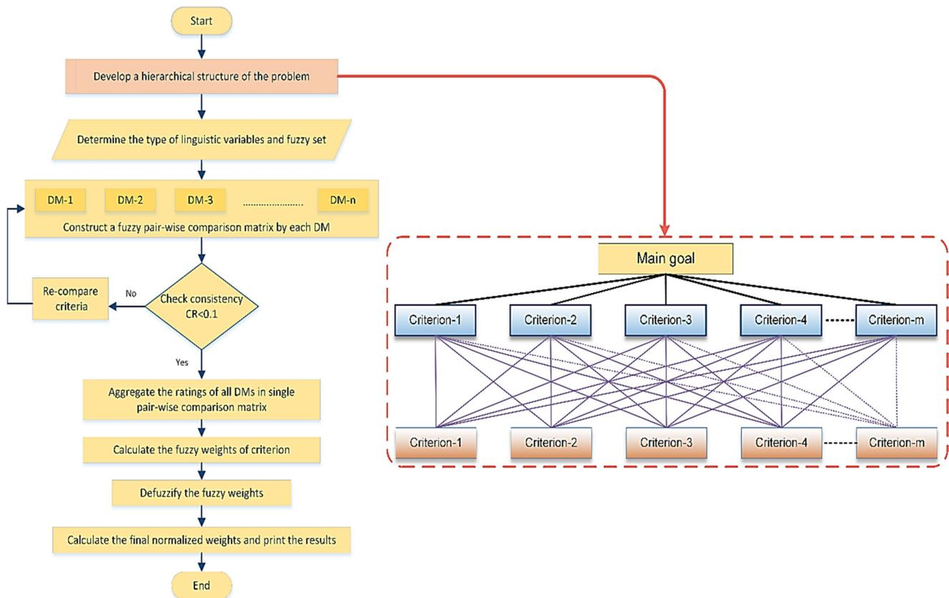
Figure 2. Flowchart of the FAHP procedure.
