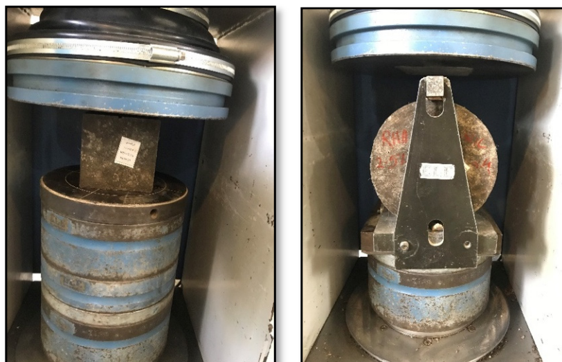
Figure 4. Tests of hardened concrete.
