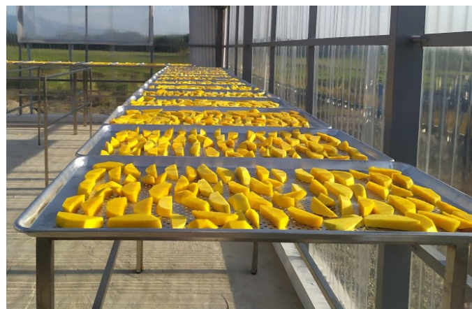
Figure 7. Mango slices in the perforated plate inside of the solar dehydrator.
