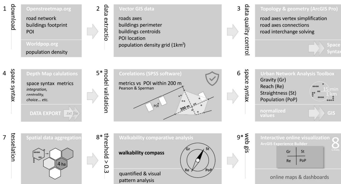
**Figure 3.** The method workflow includes spatial data download and management (step 1–3), space syntax calculations (step 4–6), walkability compass and walkability patterns analysis (step 7–8) and research outputs sharing via WebMap (step 9); stages that are subject to results reporting are marked with an asterisk.
