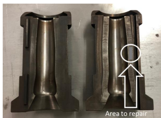
Figure 1. Case study: damaged mold for glass bottles.
