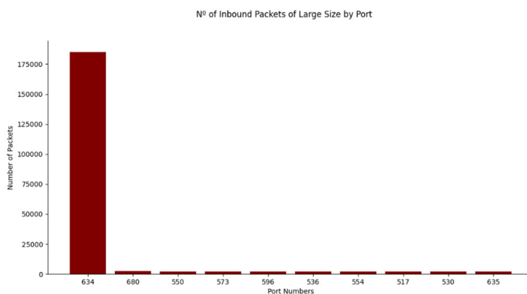
Figure 8. The number of 440-sized inbound packets, shown by port, from the NTP attack.
