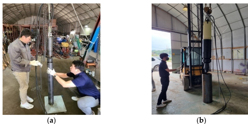
Figure 10. Comparison of developed hydraulic expansion equipment with its prototype: (a) Prototype of hydraulic expansion equipment for steel pipes with diameter of 100 mm; (b) Full-scale of hydraulic expansion equipment for steel pipes with diameter of 300 mm or more.
