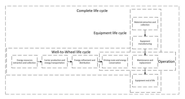
Figure 4. Basic vehicle life-cycle analysis model.
