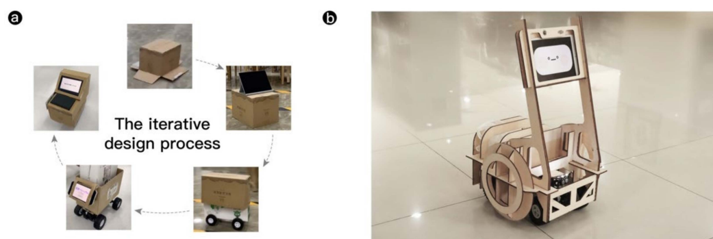
Figure 3. (a) Prototypes of previous iterations; (b) the final prototype of Anti-Sedentary Robot based on a radio control vehicle.
