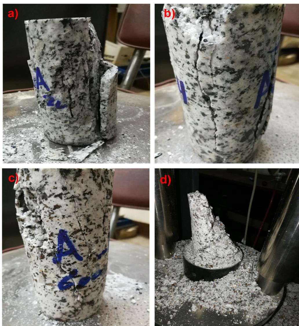
**Figure 9.** Failure modes of granodiorite samples at various thermal treatments: (a) 200 °C, (b) 400 °C, (c) 600 °C, and (d) 800 °C.
