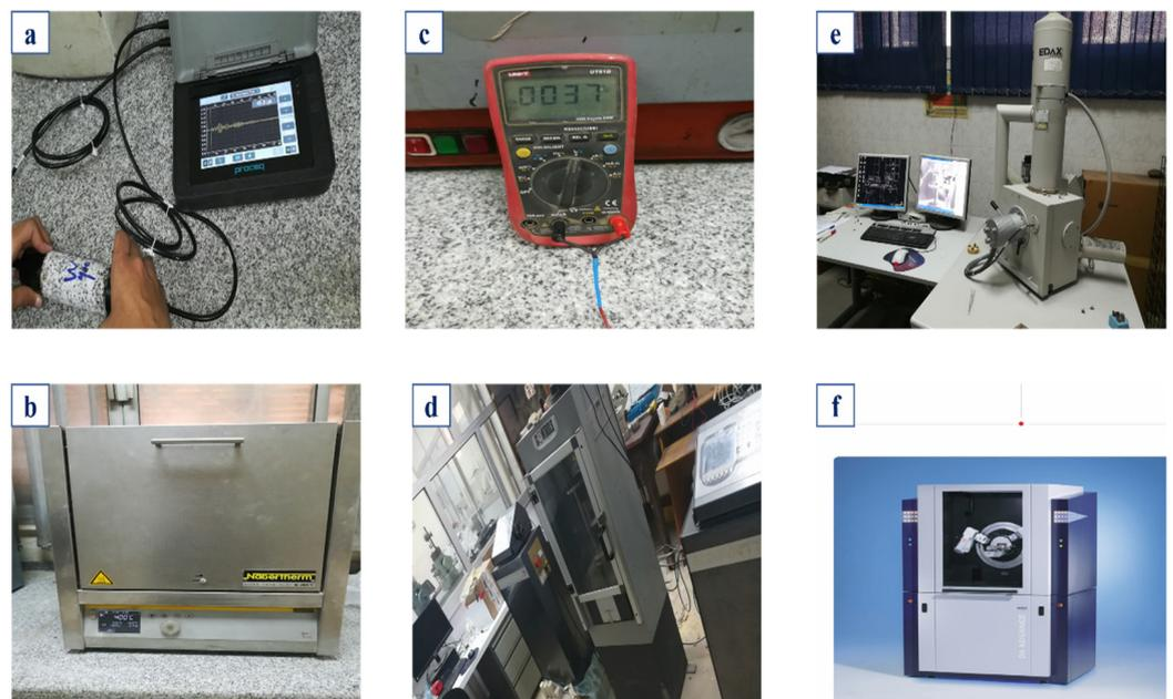
**Figure 2.** The principal used devices in this study: (a) P-wave velocity measurement tool, (b) Nabertherm electric furnace, (c) a contact thermometer, (d) uniaxial compression test machine, (e) the SEM apparatus, and (f) the XRD unit.
