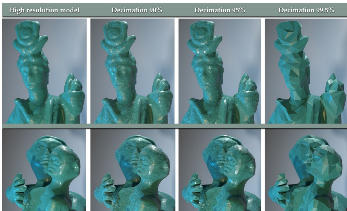
Figure 19. Examples of mesh simplification results with three levels of decimation: the Iside 3D model (middle row) decimated with Blender and the Mother with Child 3D model (bottom row) decimated with Houdini. Differences in the decimation outputs are hardly appreciable.
