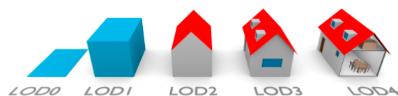
Figure 1. The five LODs of CityGML 2.0. Reprinted with permission from ref. [14]. Copyright 2016 Elsevier.
