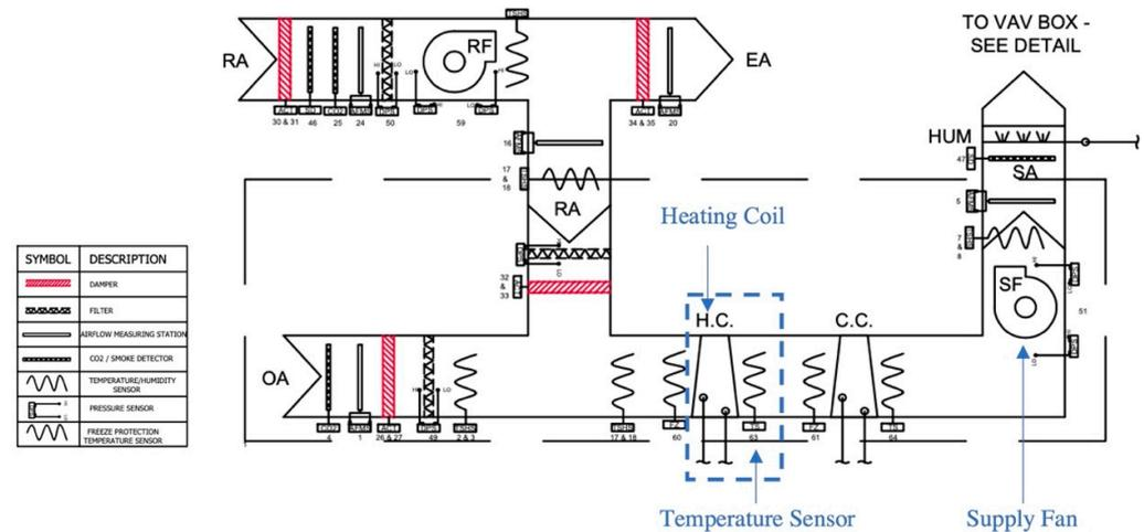
**Figure 4.** An air duct system with highlighting the heating coil, temperature sensor, and supply air fan in the image with a blur font color.
