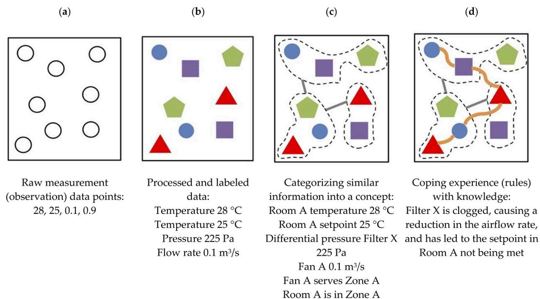
**Figure 1.** Knowledge-based fault detection of a forced air HVAC system with a clogged filter: (a) data, (b) information, (c) knowledge and (d) wisdom.
