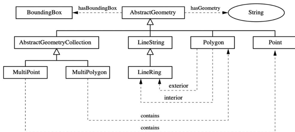
Figure 5. High-level ontology for a two-dimensional geometry and associated data and object properties [47].
