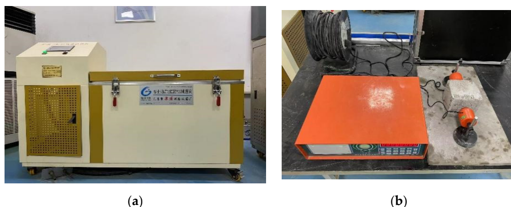
Figure 3. Test Instruments: (a) Concrete rapid freeze-thaw testing machine; (b) Concrete dynamic elastic modulus tester.
