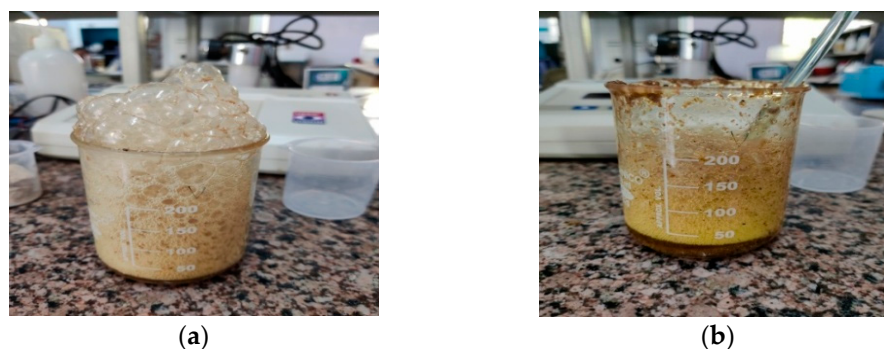
Figure 3. The foam is formed by the reaction between lime mortar and concentrated HCl solution (a) and the acidic reaction slows after a while settling down (b).
