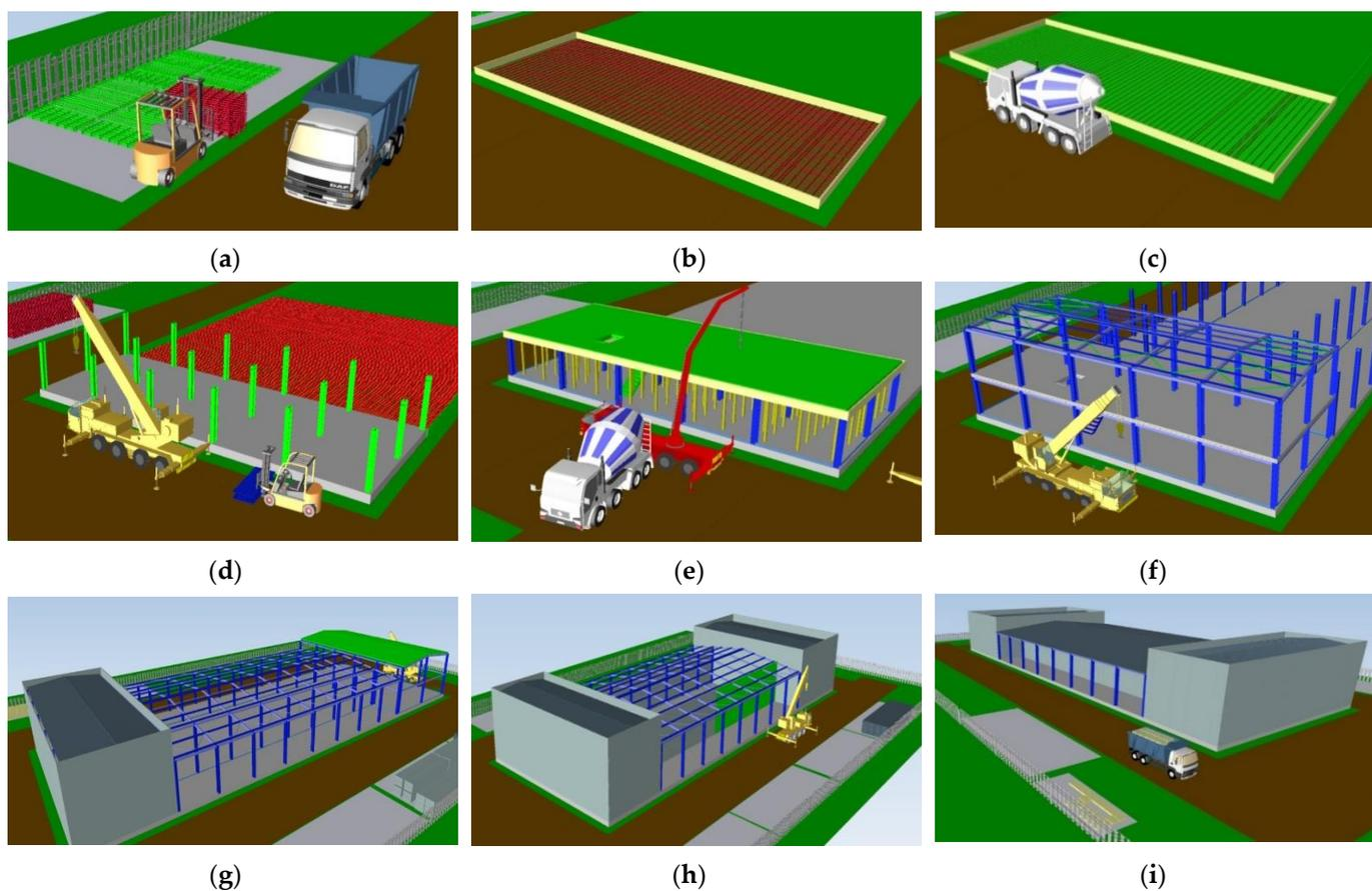
**Figure 7.** Short clips from the 4D simulation footage: (a) Reinforcement delivery and unloading; (b) Reinforcement installation (offices—foundations slab); (c) Concrete works (offices—foundations slab); (d) Columns assembly (offices—ground floor); (e) Concrete works (offices—ground floor slab); (f) Roof bracing assembly (offices—roof); (g) Roof panels assembly (warehouse); (h) Facade panels assembly (production plant); (i) Formwork removal.
