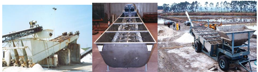
Figure 4. Examples of salt washing machines with screw conveyors [1].
