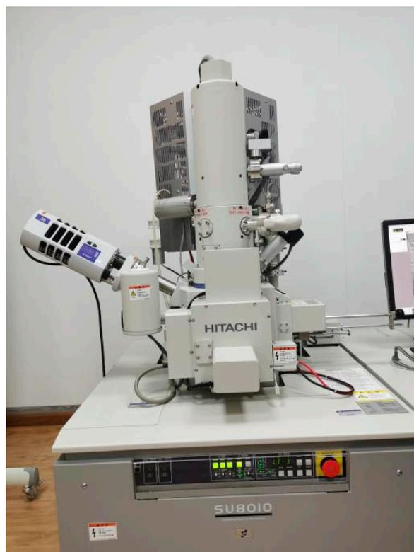
**Figure 4.** SU8010 high resolution field emission scanning electron microscope.
