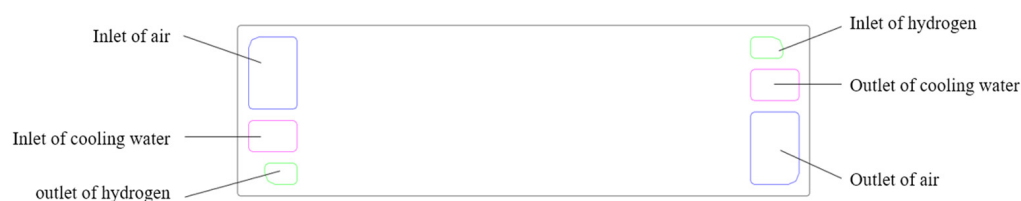
Figure 7. Inlets and outlets of cooling water in the BPP to warm up the fuel cell stack.
