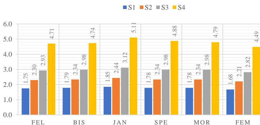
Figure 18. FoS for Slope 1:1, H = 3.00 m, S1–S4.
