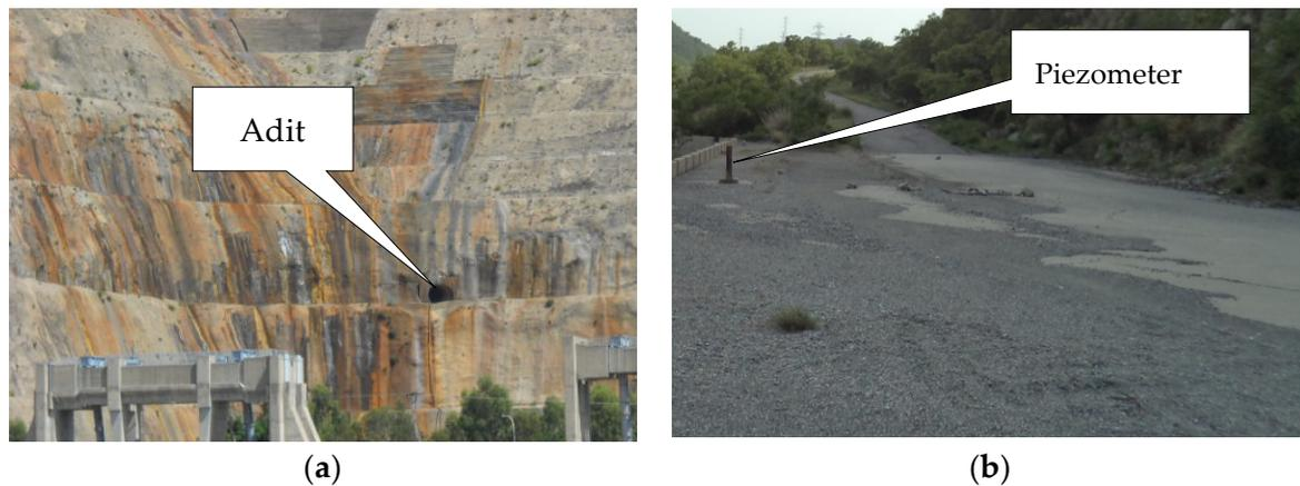
**Figure 4.** Study area details observed during reconnaissance. (a) View of an adit shown in cut slopes. (b) Piezometer installed.
