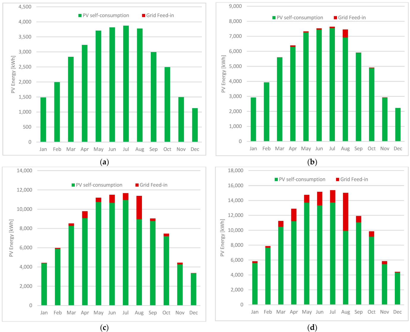
Figure 8. Use of PV energy for (a) 25.2 kW, (b) 50 kW, (c) 75.6, and (d) 100 kW PV systems. The horizontal axis is time (month).
