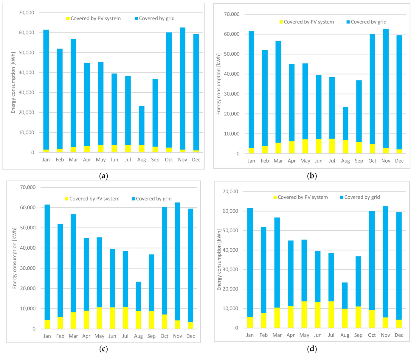
Figure 7. Electricity consumption coverage for (a) 25.2 kW, (b) 50 kW, (c) 75.6, and (d) 100 kW PV systems. The horizontal axis is time (month).
