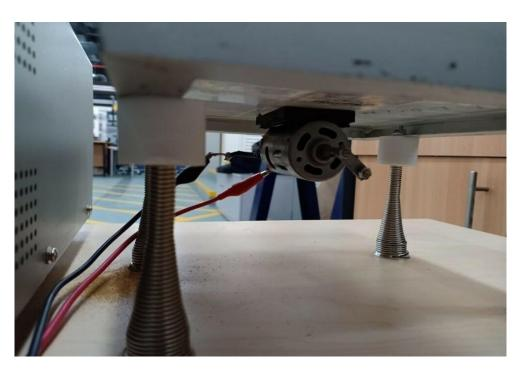
Figure 6. DC motor attached to solar panel rear for vibration cleaning [55].
