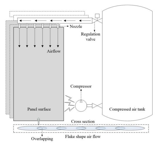
Figure 7. Regulatory mechanism for solar PV panel arrays using compressed air [37].
