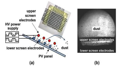
**Figure 4.** The electrostatic cleaning procedure Some dust particles pass through the hole in the upper screen electrode due to their inertia force and the alternating electrostatic field near the electrodes stirs up the dust particles, and a high-speed microscope camera was used to capture the results as shown in (**a**) and (**b**) respectively [49].
