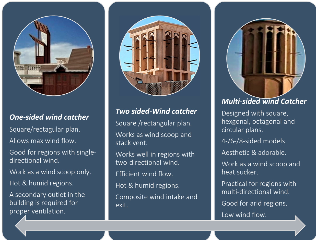
Figure 3. Elements of wind catcher design and performance Source [76].
