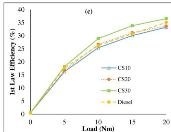
Figure 2. 1st law efficiency of primary biodiesel blends in comparison with diesel for (a) palm, (b) jatropha and (c) cottonseed blends.
