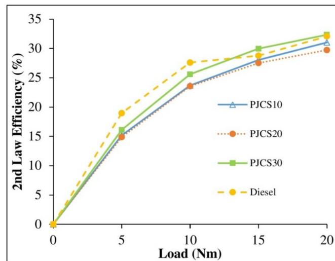
**Figure 7.** 2nd Law Efficiency of ternary biodiesel blends in comparison with diesel.
