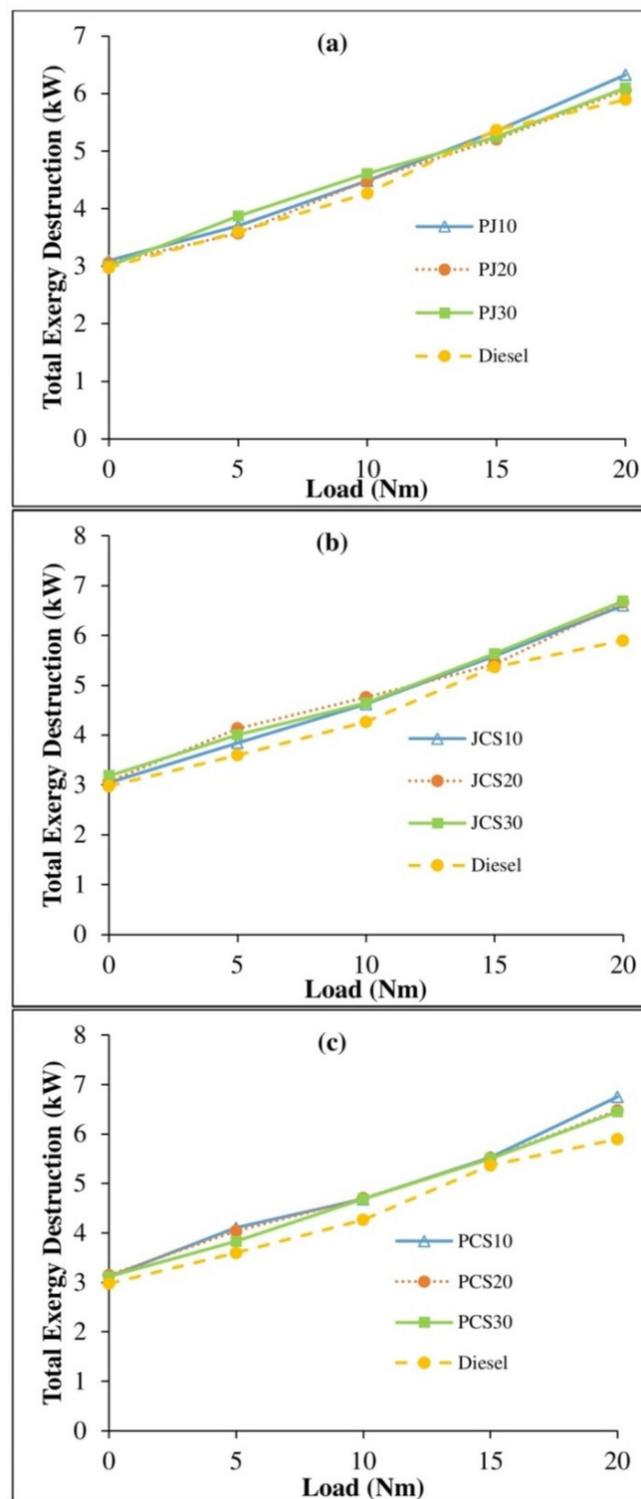
**Figure 12.** Total exergy destruction of binary biodiesel blends in comparison with diesel for (a) palm-jatropha, (b) jatropha-cottonseed and (c) palm-cottonseed blends.
