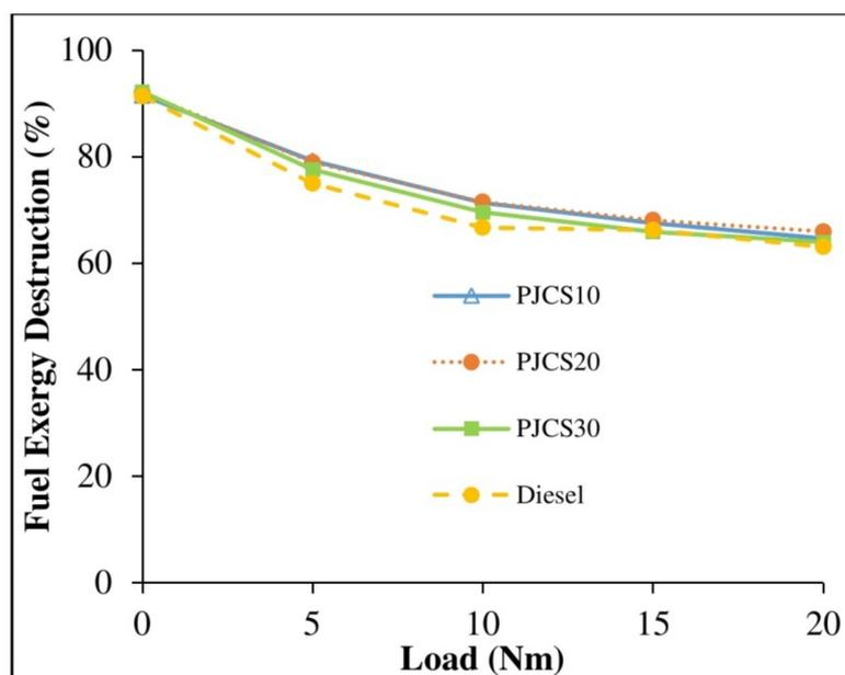
**Figure 10.** Fuel exergy destruction of ternary biodiesel blends in comparison with diesel.
