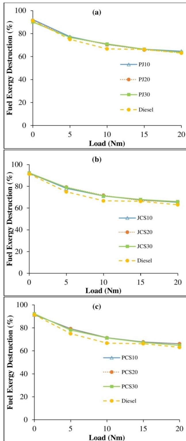
Figure 9. Fuel exergy destruction of binary biodiesel blends in comparison with diesel for (a) palm-jatropha, (b) jatropha-cottonseed and (c) palm-cottonseed blends.
