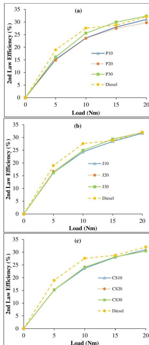
**Figure 5.** 2nd law efficiency of primary biodiesel blends in comparison with diesel for (a) palm, (b) jatropha and (c) cottonseed blends.
