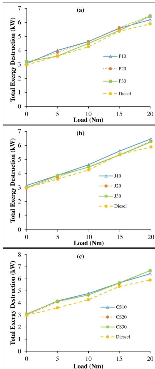
Figure 11. Total exergy destruction of primary biodiesel blends in comparison with diesel for (a) palm, (b) jatropha and (c) cottonseed blends.
