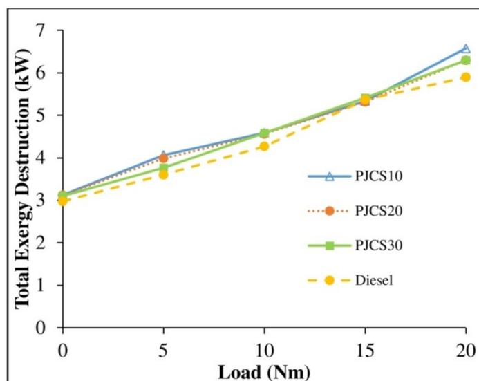
Figure 13. Total exergy destruction of ternary biodiesel blends in comparison with diesel.
