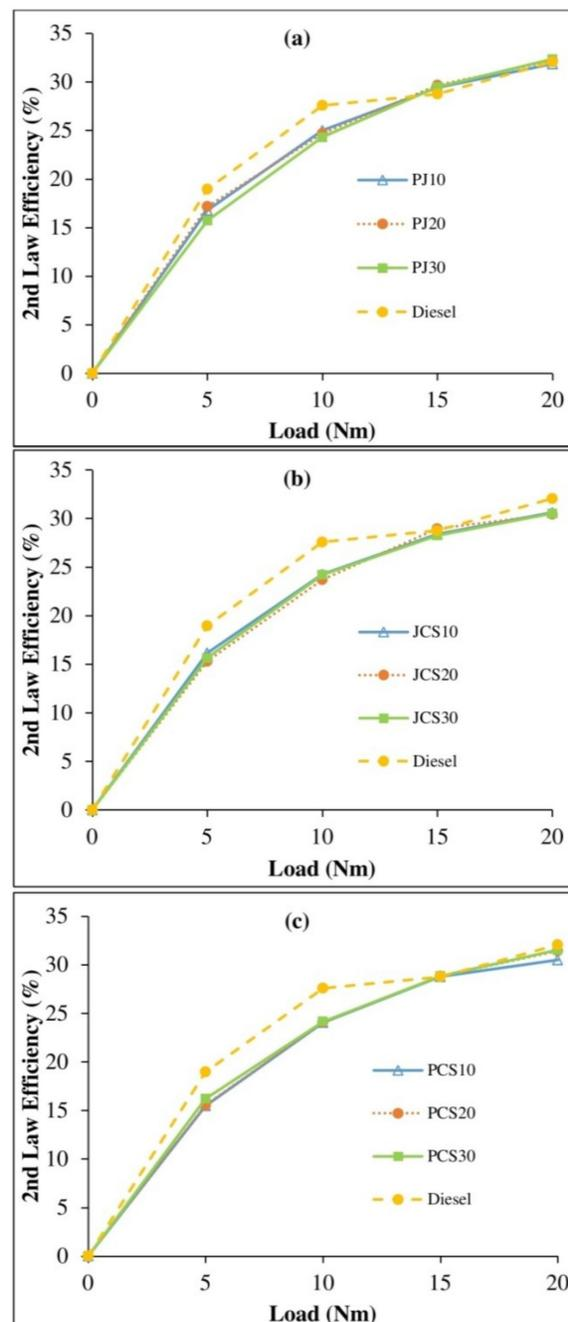
**Figure 6.** 2nd law efficiency of binary biodiesel blends in comparison with diesel for (a) palm-jatropha, (b) jatropha-cottonseed and (c) palm-cottonseed blends.
