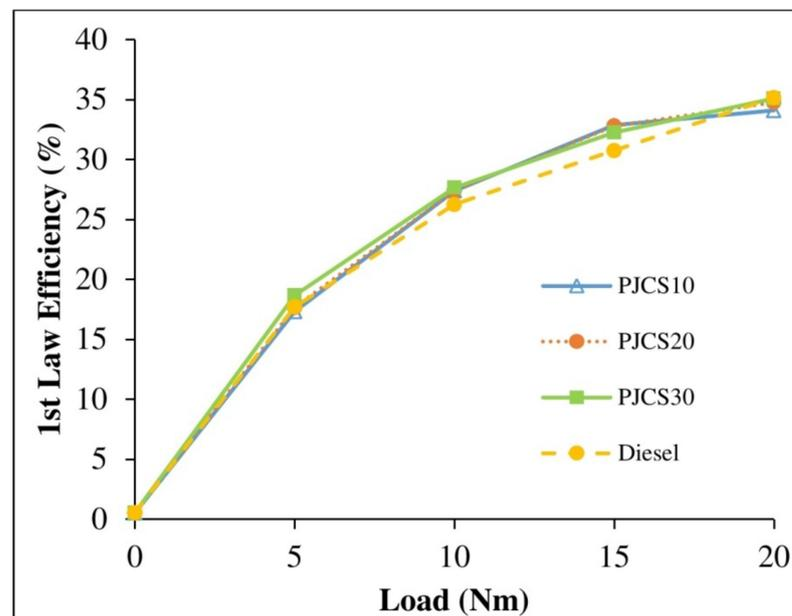
**Figure 4.** 1st law efficiency of ternary biodiesel blends in comparison with diesel.
