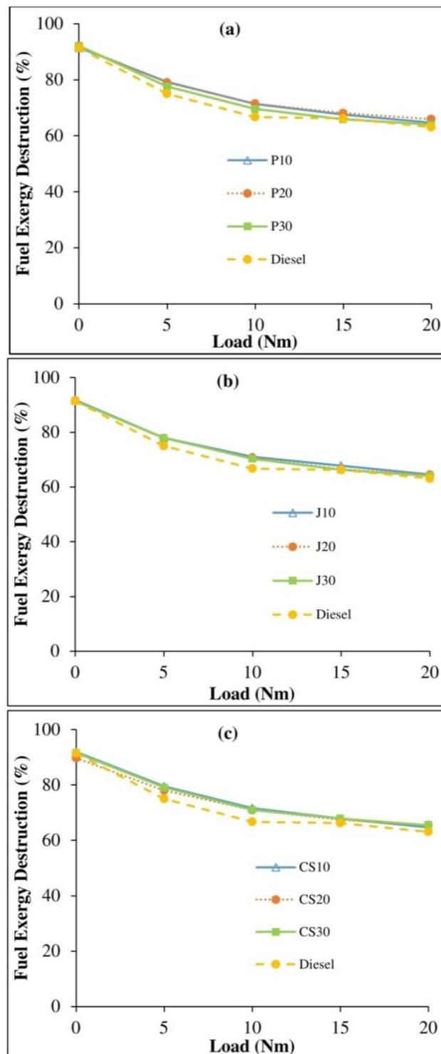
**Figure 8.** Fuel exergy destruction of primary biodiesel blends in comparison with diesel for (a) palm, (b) jatropha and (c) cottonseed blends.
