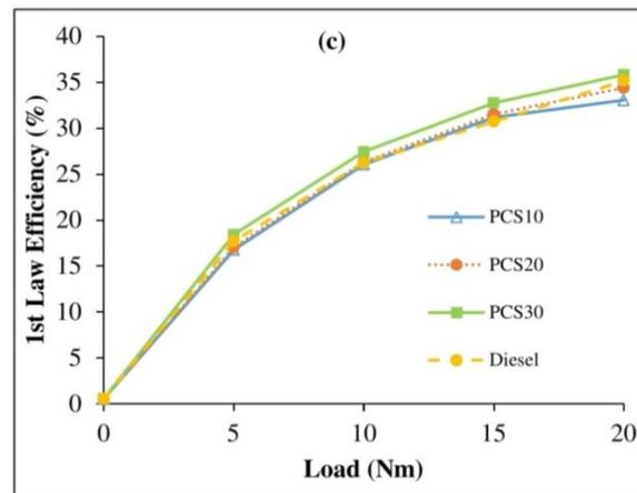
**Figure 3.** 1st law efficiency of binary biodiesel blends in comparison with diesel for (a) palm-jatropha, (b) jatropha-cottonseed and (c) palm-cottonseed blends.
