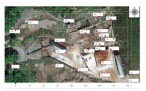
Figure 4. Site layout, (red points are locations or reading stations).
