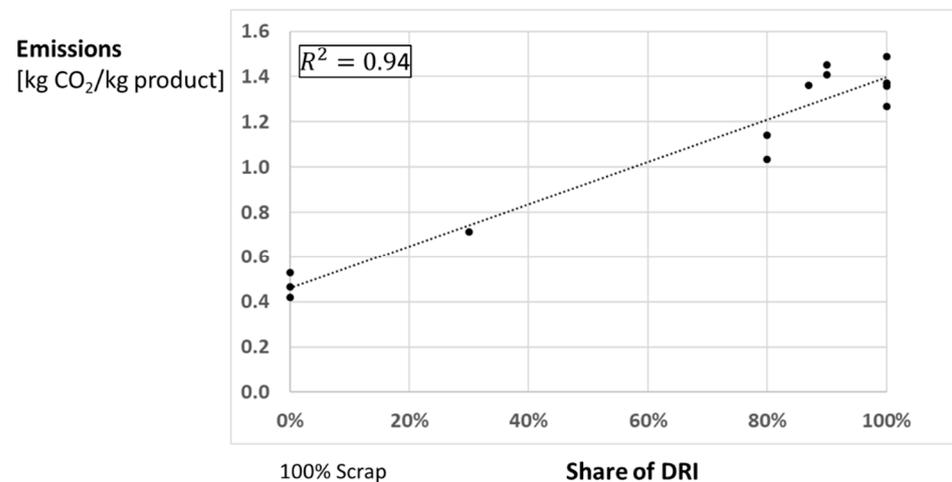
**Figure 7.** Carbon dioxide emissions of steel and hot-rolled coil production via a natural gas-based direct reduction (DR) plant combined with electrical melting. The emissions are presented as a function of a combined scrap and direct reduced iron (DRI) melting (kg DRI/(kg DRI + kg scrap)) [29,74–77,80,82].
