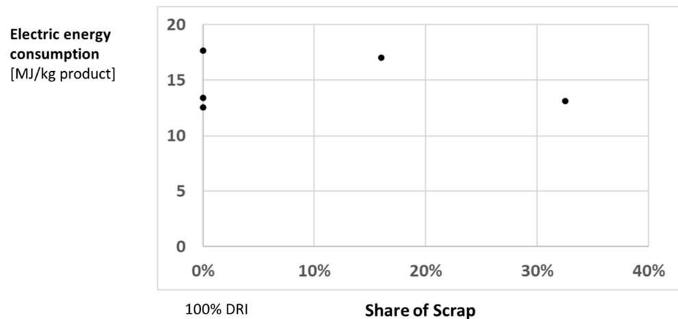
**Figure 9.** Electric energy consumption of steel and hot-rolled coil production via a hydrogen-based direct reduction (DR) plant combined with electrical melting. The energy consumption is presented as function of a combined scrap and direct reduced iron (DRI) melting (kg scrap/kg product) [74,82,83,86,87].
