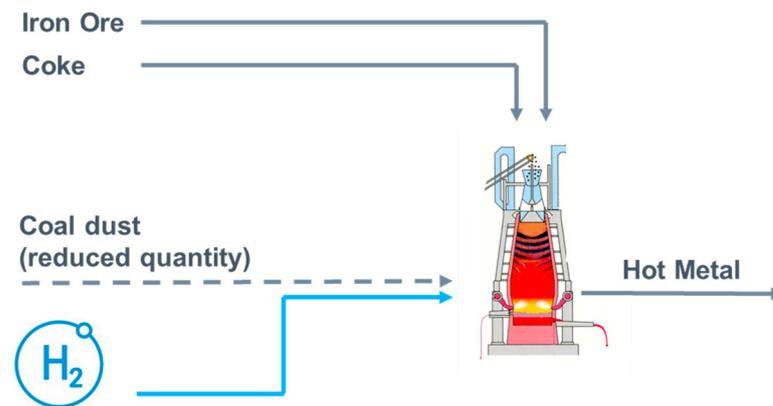
**Figure 3.** Injection of hydrogen into a blast furnace.
