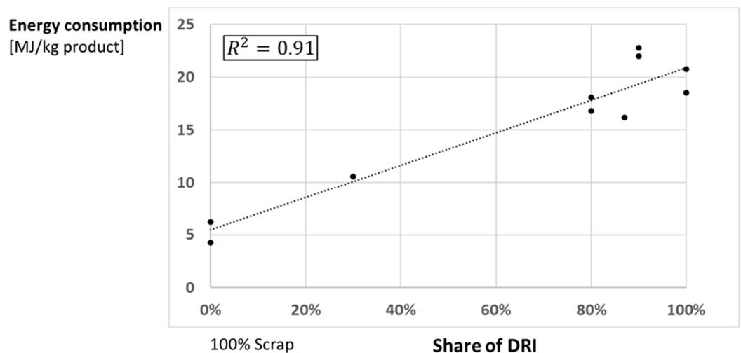
**Figure 8.** Energy consumption of steel and hot-rolled coil production via a natural gas-based direct reduction (DR) plant combined with electrical melting. The energy consumption is presented as a function of a combined scrap and direct reduced iron (DRI) melting (kg DRI/(kg DRI + kg scrap)) [74–77,80].
