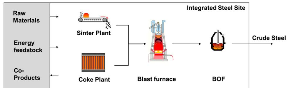
**Figure 1.** System boundary of an integrated steel site.
