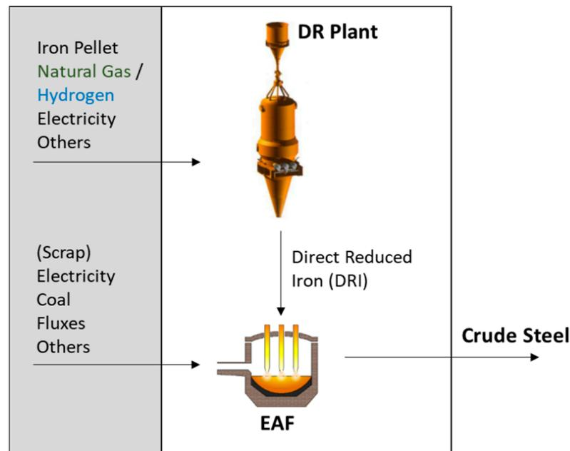
**Figure 6.** System boundary of crude steel production via a direct reduction plant (DR) and an electric arc furnace (EAF). Both, natural gas and hydrogen can be used as reducing agent within the DR plant.
